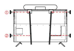
B When the screen is mounted on the TV Mount brackets
